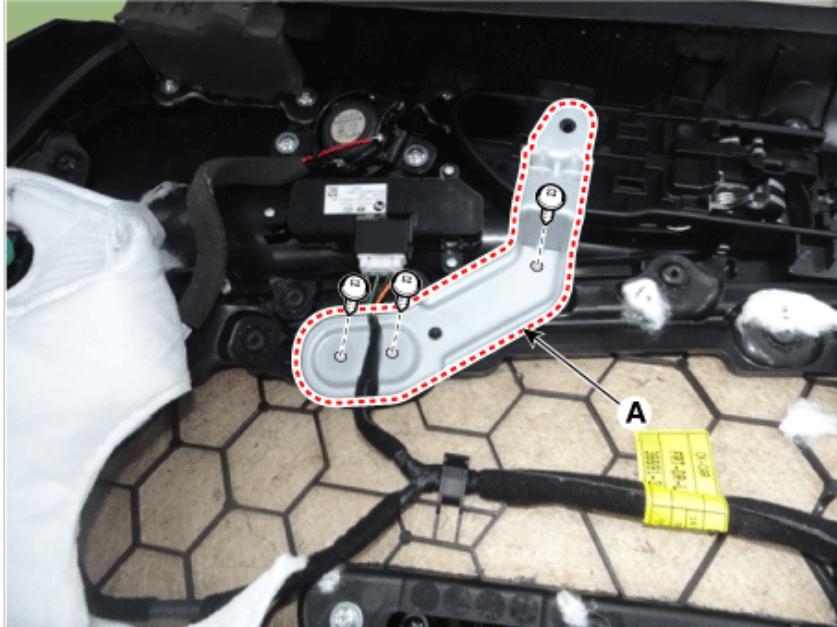
3. Remove the front door inside handle (A) after loosening mounting screws.
